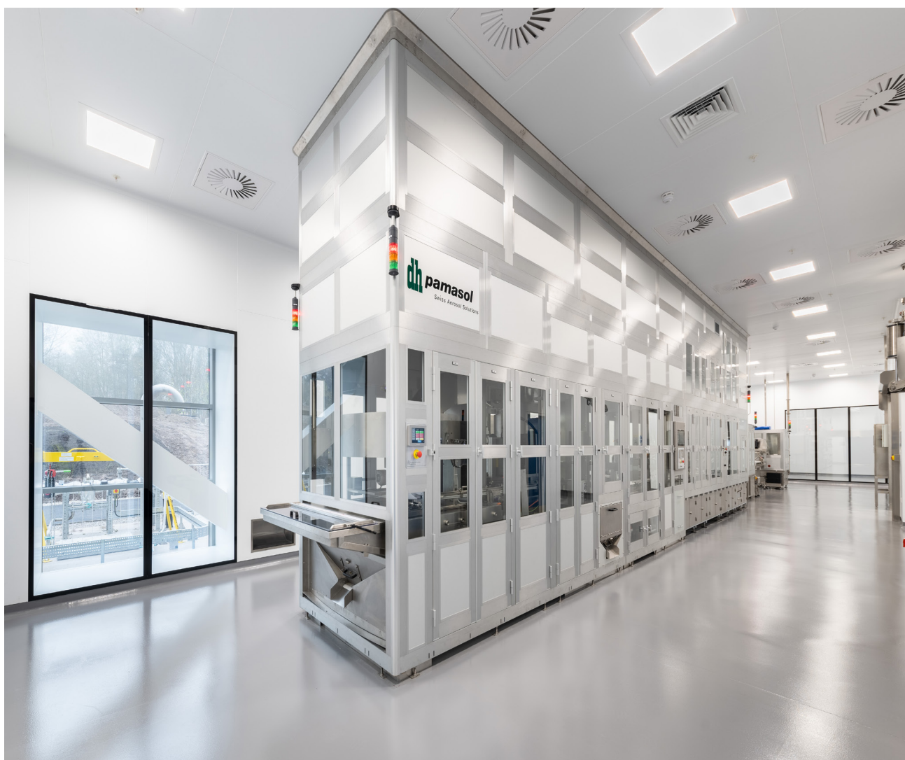
Figure 1: Bepak's line 3, focused on the production of low Global Warming Potential (GWP) propellants HFA-152a and HFO-1234ze.
